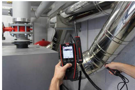
Hygrometry and air velocity measurement
